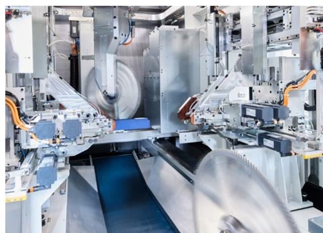
Vertical and horizontal sawing units for complex cutting, notching and combinations
