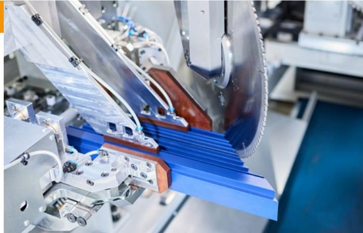
2 separate servo vertical clamps for optimum clamping
