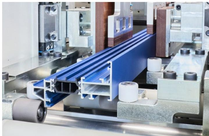
Guiding elements and clamps adapted to complex window sash profile
