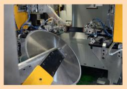
Saw Module "SUA 1" - 4 CNC-axes for each best approach angle - integrated Micro-Spraying Unit for cooling
